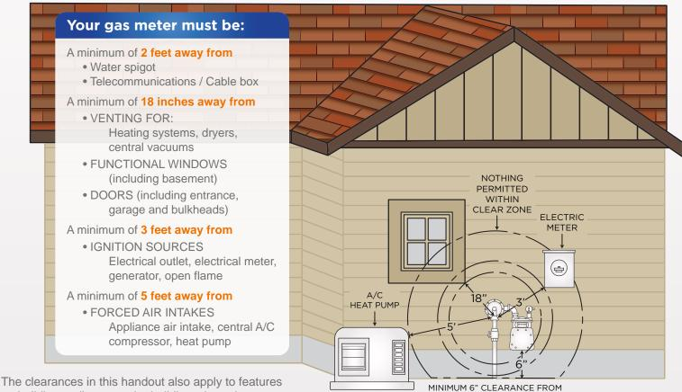
The clearances in this handout also apply to features on buildings adjacent to the building where the gas meter is located.
